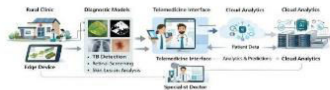
Fig.1. Architecture of an AI-driven rural healthcare system integrating diagnostic models, telemedicine interface, cloud analytics, and edge computing devices.
